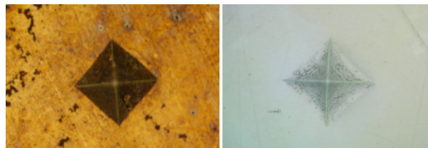
Fig. 2. Example of different contrast images for imprints on materials: copper on the left, polycarbonate on the right
